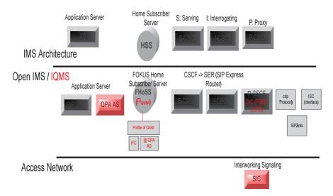
Figure 14. Architecture IMS versus IMS-IQMS
