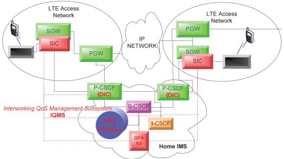
Figure 4.Introducing management components into IMS: SICs, DIC and HSS-PQoS<sub>R</sub>
