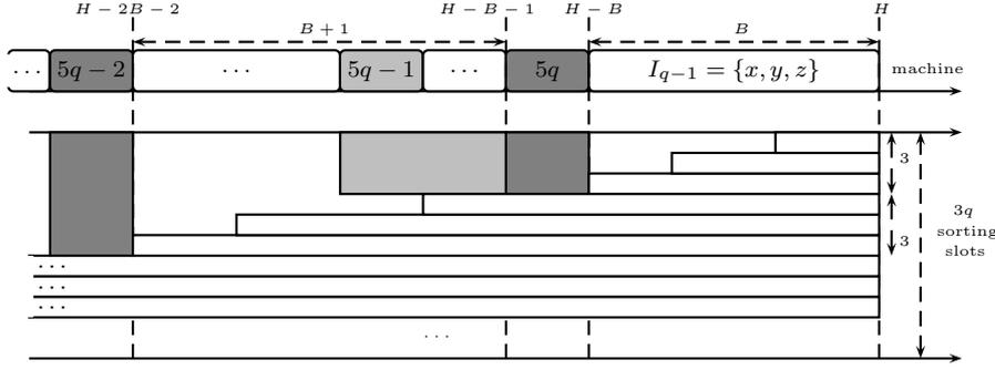
**Fig. 4** Reducing the 3-PARTITION problem to the sorting slot problem (the part above the time-axis represents the schedule of jobs on the machine, while the part below represents the use of the sorting slots over the time horizon). **Case of  $I_{q-1}$**
