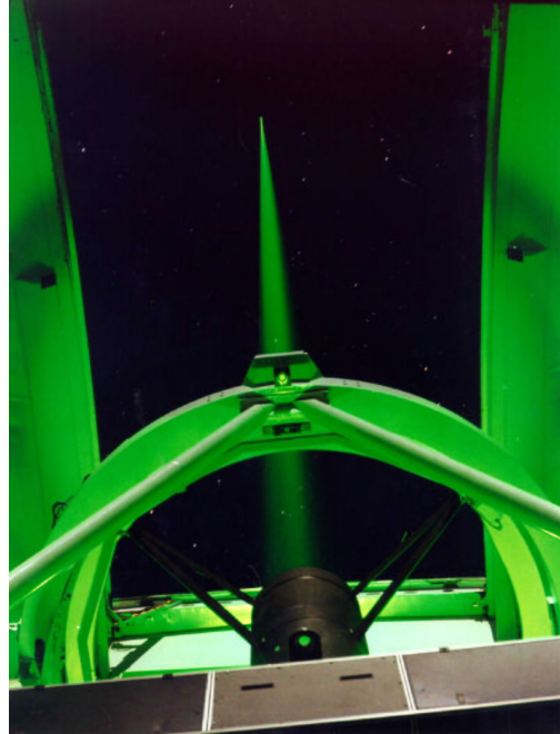
Figure 27: The laser beam emitted from the 4.2m WHT telescope. The backscattered LGS is selected at \approx 20\text{km} where the beam is focused.
