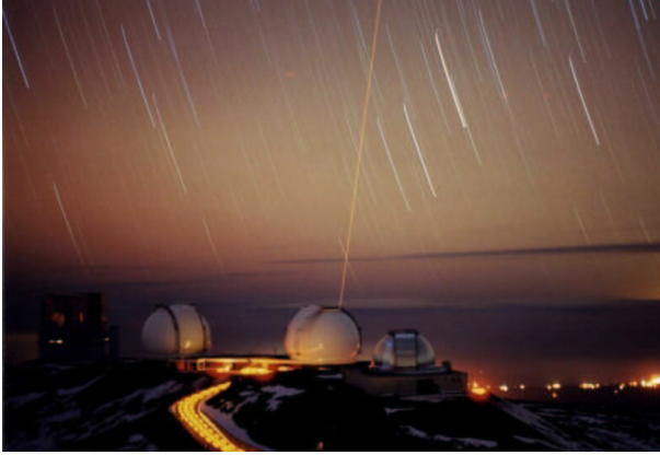
Figure 32: The laser beam emitted by the 10m Keck-II telescope at the top of the 4200m high Mauna Kea sleeping volcano in Hawaii. It is taken 600m away, from the Canada-France-Hawaii (CFHT) telescope. One sees the faint Mie + Rayleigh scattering, as well as the star trails in the sky due to the diurnal motion of the stars during the 20 mn exposure. Hazard lights from a vehicle mark the steep descent path of the summit. Photo credit: John McDonald, CFHT Corp.
