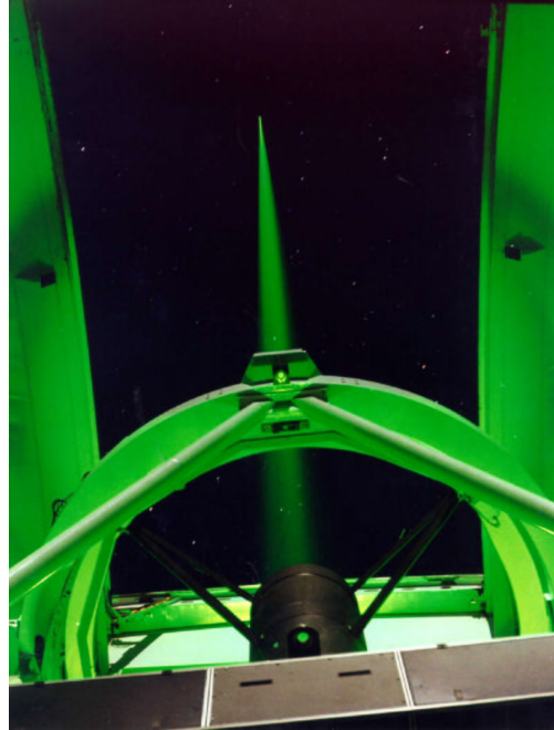
Figure 27: The laser beam emitted from the 4.2m WHT telescope. The backscattered LGS is selected at \approx 20 km where the beam is focused.
