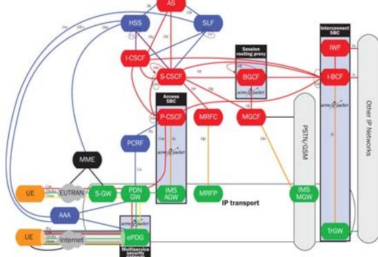
Figure 1: IMS Design as defined in 3GPP IMS Release 8 [19]
