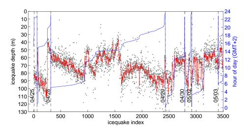
Figure 6: Icequakes depths (dots) and median values for a sliding window of 10 events (red), for all icequakes of cluster B with peak amplitude  $A > 300 \ \mu m/s^2$  and correlation  $C \ge 0.7$ . The blue line indicates the hour of the day (local time), and each vertical dashed line indicates a new day.
