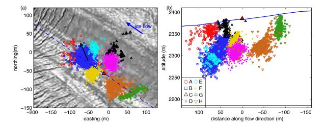
Figure 5: (a) Map of the icequakes for all of the events with peak amplitude  $A > 300 \ \mu m/s^2$ ,  $\phi < \phi^*$  and correlation  $C \ge 0.7$ . For cluster *B*, the black arrow shows the dip direction. (b) Cross-section in the glacier flow direction. The blue line shows the ice surface along the dashed blue line shown in (a), and the black line indicates the ice/rock interface. The seismic sensor is shown by a red triangle.
