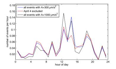
Figure 8: Diurnal distribution of the icequakes for different amplitude thresholds:  $A > 300 \ \mu m/s^2$  (blue, red) or  $A > 1000 \ \mu m/s^2$  (black). Times are local (Greenwich Mean Time +2 h). The strong peak at 14:00 disappears when events that occurred on 4 April were excluded (red).
