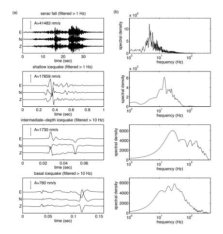
Figure 2: (a) Waveforms and (b) Fourier transform for the different types of events. The signals were converted to ground velocity and high-pass filtered. Note the different time scales for the waveforms.
