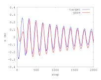
Fig. 7. Target and gaze alongside the  $\boldsymbol{x}$  axis during an oscillation frequency of 0.6Hz.
