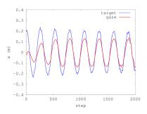
Fig. 8. Target and gaze alongside the  $\boldsymbol{x}$  axis during an oscillation frequency of 0.4Hz with clamped joints.
