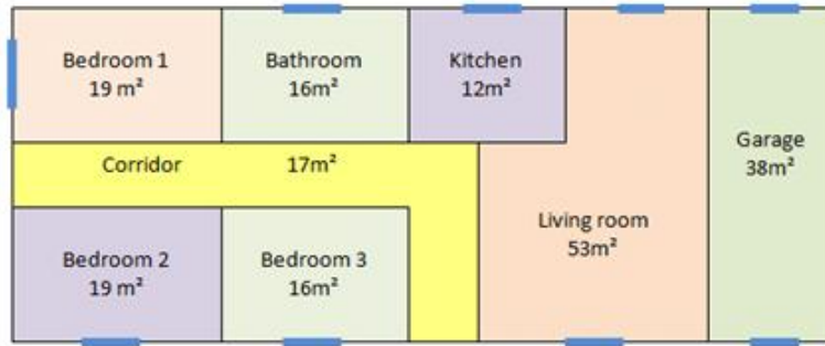
Figure 3: Plan of the 150 m 2 single-storey house. Windows are represented in blue
