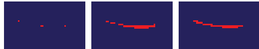
Figure 13: Footprint of a B-Rep surface tessellated into a set of triangles, rendered by the GPU. Left: filled polygon mode. The fragments affected by the rasterization leave a discontinuous footprint on screen, as only 4 fragments have their centerpoint actually lying within the boundaries of the tessellated primitives. The rendering obtained is illustrated in Figure 10. Middle: 4x multisampling. The footprint left out by the surface on the screen still is non-continuous. Right: wireframe mode provides a suitable result.
