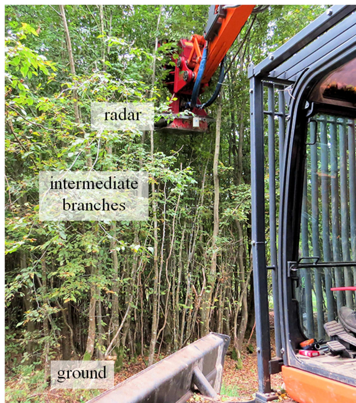
Fig. 8. General view of the experiment realized in the forest. The radar must be able to detect the ground even if obstacles such as branches or bushes are present.
