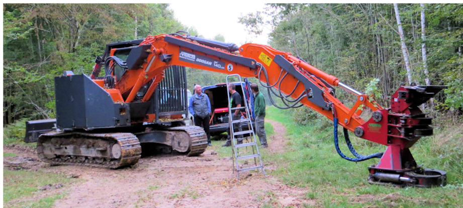
Fig. 6. General view of the hydraulic excavator used during the experiments in the forest. The excavator is equipped with a shear cutting head from VIGNEAU Society.
