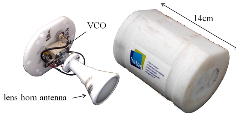
Fig. 4. LFM CW radar integration. Left: the microwave VCO is equipped with a lens horn antenna. Right: transparent to radar waves, the radome is a mechanical protection for the radar.
