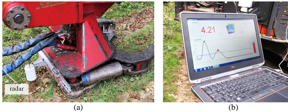
Fig. 7. Positioning of the equipment. (a) Rear position of the radar, fixed on the shear cutting head. (b) A graphical interface on the laptop allows to control the process.
