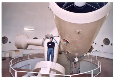
Fig. 5. The 2 pendular seismometers (Tokovinin 2000) mated to the OHP 1.5m telescope for vibration measurements simultaneously with differential tip tilt ones.
