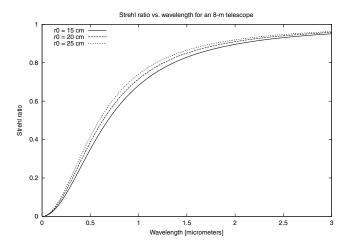
**Figure 7.** Maximum Strehl ratio versus wavelength for values of  $r_0$  ranging from 15 to 25 cm for the 8-m configuration denoted '8-m II' in Table 1. Optimal integration times range from 20 ms ( $r_0 = 15$  cm) to 26 ms ( $r_0 = 25$  cm).
