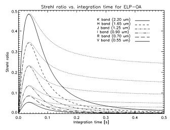
**Figure 4.** Strehl ratio versus integration time for several astronomical observation bands for the configuration denoted 'ELP-OA II' in Table 1 and  $r_0 = 10$  cm. Solid and dashed lines, high-bandwidth approximation; dotted lines, exact solution. The optimal integration time,  $t_{\text{i.max}}$ , is 35 ms.
