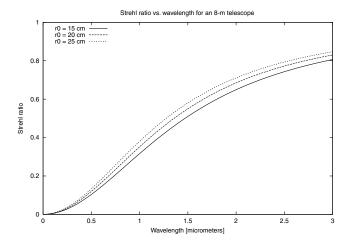
**Figure 6.** Maximum Strehl ratio versus wavelength for values of  $r_0$  ranging from 15 to 25 cm for the 8-m configuration denoted '8-m I' in Table 1. Optimal integration times range from 42 ms ( $r_0 = 15$  cm) to 56 ms ( $r_0 = 25$  cm).
