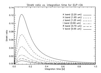
**Figure 2.** Strehl ratio versus integration time for several astronomical observation bands for the original configuration of ELP-OA ('ELP-OA I' in Table 1) and  $r_0 = 10$  cm (at 0.5  $\mu$ m). The high-bandwidth approximation was used to calculate these results. The optimal integration time,  $t_{i,max}$ , is 92 ms.
