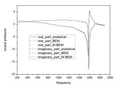
FIGURE 3 – Pressure at right imaginary end of straight pipe
