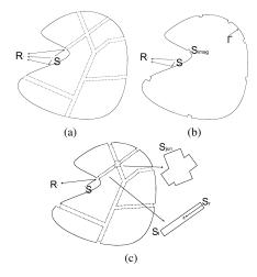
FIGURE 1 – (a) Total pressure ; (b) Pressure directly from source and reflected by flange ; (c) Pressure radiating from network
