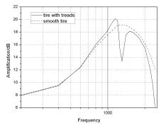
FIGURE 10 - Comparison of amplification of horn effect
