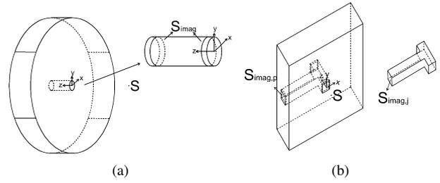
FIGURE 2 – (a) One pipe with cylindrical flange ; (b) T pipe with rectangular flange.
