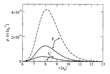
FIG. 7. Comparison of radial helium density profiles obtained with HCN rotation (solid lines) and without HCN rotation (dashed lines) along the privileged axes F ( $\theta$ =0) and U ( $\theta$ = $\pi$ ) for HCN–He.
