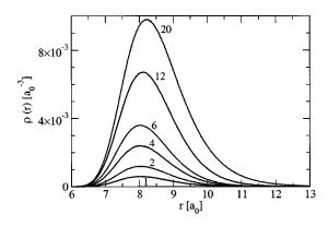
FIG. 11. Integrated radial density profiles for  $SF_6-He_N$ , N = 1,2,4,6,12,20. All profiles exhibit a single peak that grows with N, showing that the first solvation shell is still being filled for  $N \le 20$ . Reference 40 contains profiles for larger clusters sizes having additional shells populated.
