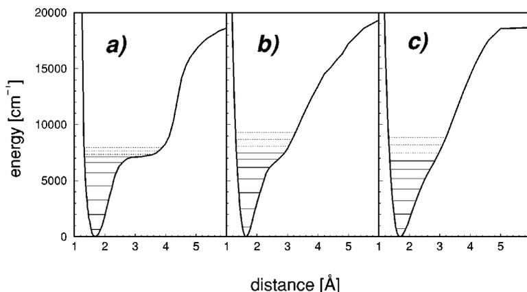
FIG. 3. Potential energy curve for the  $A\ ^1\Sigma^+$  state of AgH: (a) constructed graphically by Learner (Ref. 3), (b) calculated using SO-MCQDPT with the CAS-*a* state-specific orbitals, and (c) calculated using SO-MCQDPT with the state-averaged orbitals. Vibrational levels for each curve are obtained by numerical integration. Levels printed with dotted line were not observed in experiment.
