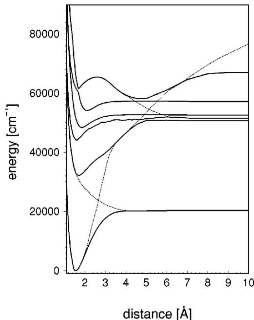
FIG. 1. Six lowest  $0^+$  states obtained from the SO-MCQDPT calculation using the state-averaged orbitals. Avoided crossings responsible for the unusual shape of the  $A^1\Sigma^+$  potential are plotted schematically using dotted lines. The dissociation limit corresponding to  $\text{Ag}^+\text{H}^-$  (the highest dotted line) is out of the range of this plot.
