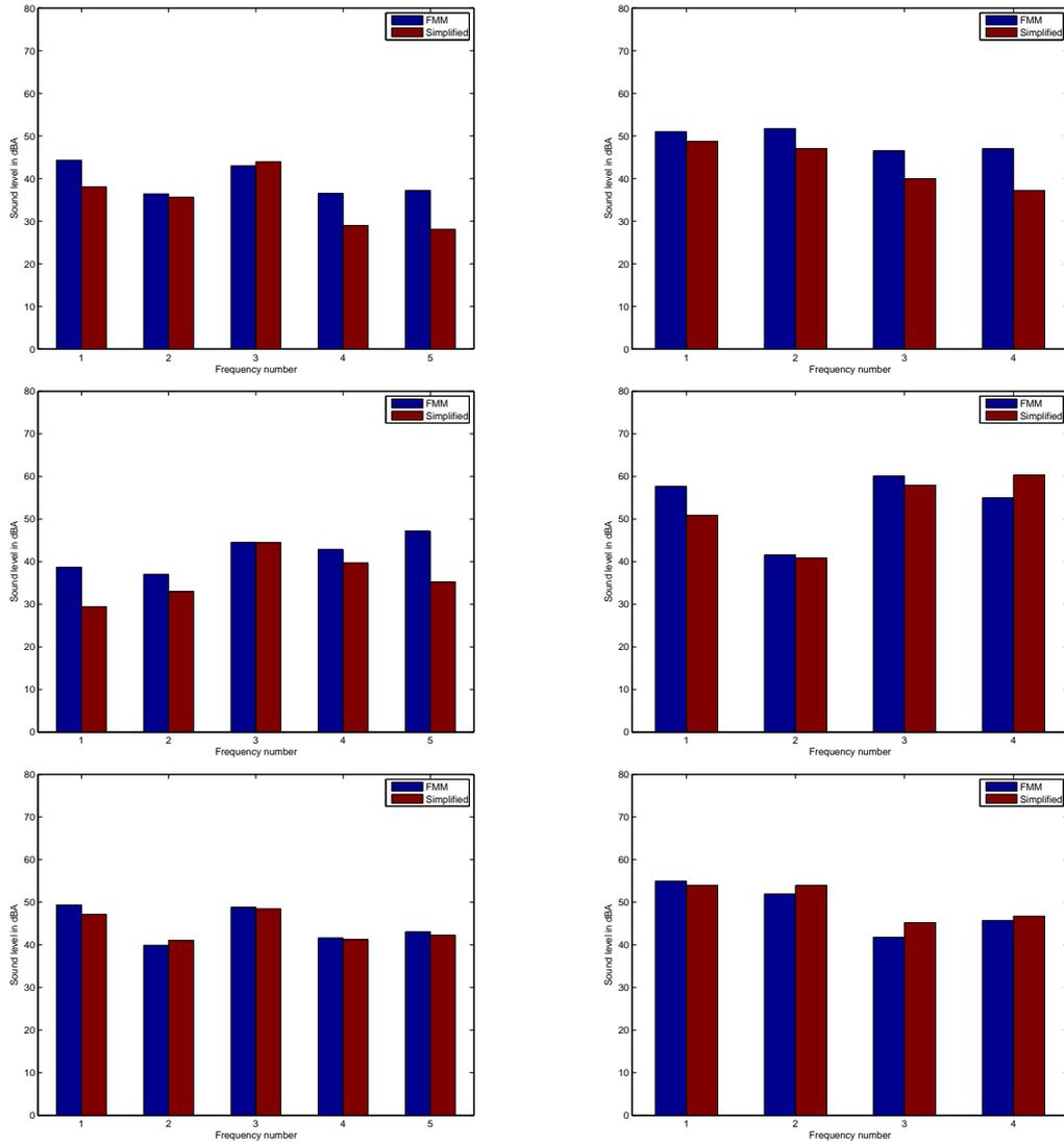
**Figure 7:** Sound level at point 1 (upper figure), point 2 (middle figure) and point 3 (bottom figure) for the disc (left figures) and the caliper (right figures)
