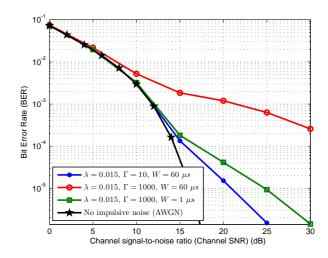
Figure 4. BER performance for two different values of each of  $\Gamma$  and W while keeping the other parameters constant.
