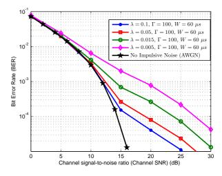
Figure 3. BER performance for different values of  $\lambda$  and for  $\Gamma = 100$  and  $W = 60 \ \mu s$ .
