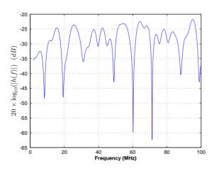
Figure 1. Simulated PLC channel transfer function.
