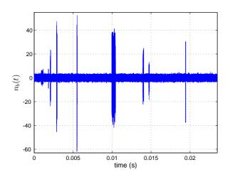
Figure 2. Impulsive noise model with  $\lambda = 0.005 \ s, \Gamma = 100$  and  $W = 100 \ \mu s.$
