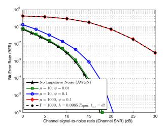
Figure 5. BER performance using BG noise model with different values of model's parameters.
