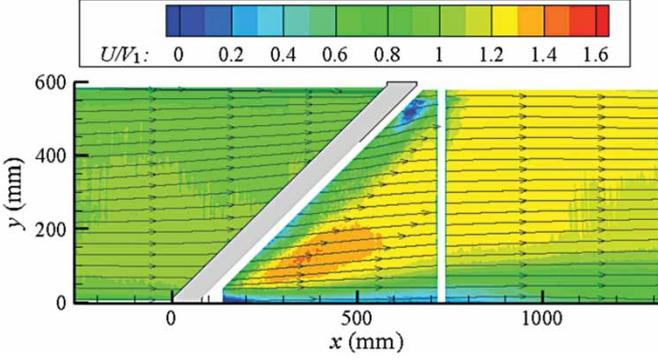
Figure 3 Velocity distribution around  $\alpha$ -SB racks with  $\alpha = 45^\circ$ .  $U/V_1$  fields are calculated from PIV measurements. Bars are rectangular and  $e = 10$  mm. The dark blue area at the downstream end of the rack is a zone of poor correlation caused by air bubbles reflecting the laser beam
