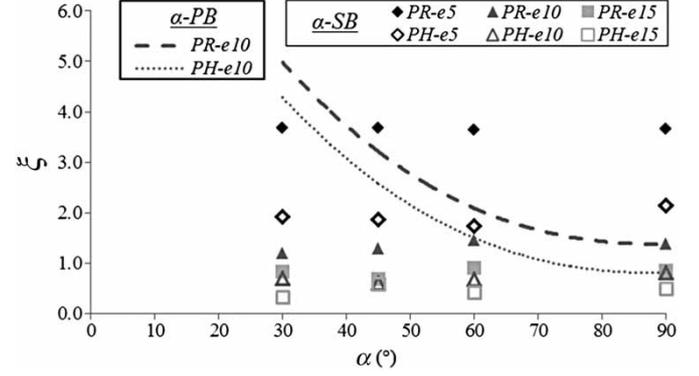
Figure 2 Head-loss coefficient  $\xi$  values for  $\alpha$ -SB racks (marks) for different bar spacings (model dimensions). Values for  $\alpha = 30^\circ, 45^\circ$  and  $60^\circ$  are those measured in this study. The  $\xi$  values at  $\alpha = 90^\circ$ , the dashed line (PR) and the dotted line (PH), illustrating  $\alpha$ -PB head-loss coefficients for  $e = 10$  mm, are extracted from Raynal *et al.* (2013)
