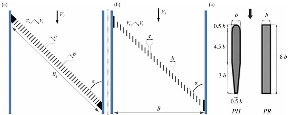
Figure 1 Comparative diagrams for (a)  $\alpha$ -PB and (b)  $\alpha$ -SB racks. (c) The two bar sections tested (PH and PR) are also detailed
