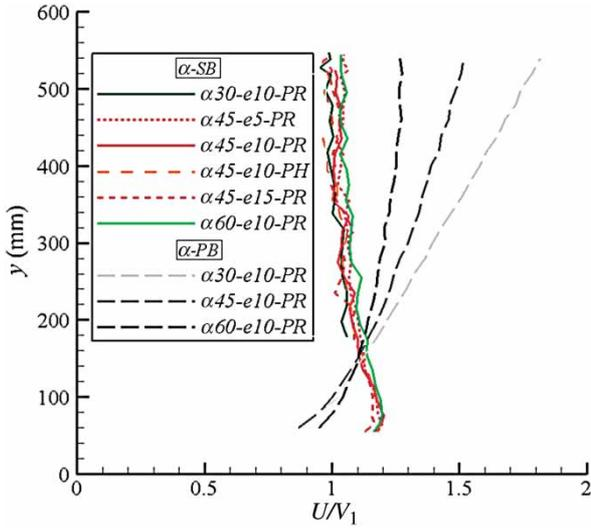
Figure 4 Comparison between velocity distributions obtained by Raynal *et al.* (2013) along  $\alpha$ -PB racks with those measured in this study along  $\alpha$ -SB racks with various angles  $\alpha$ , bar shapes and bar spacings  $e$ . Velocities are measured with an ADV probe at 50 mm upstream of the rack. The component  $U$  is normalized by the upstream mean velocity  $V_1$
