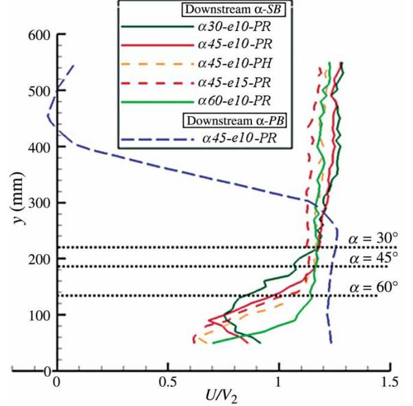
Figure 5 Transverse velocity distributions (ADV at  $x = 1 \text{ m}$ ) downstream of  $\alpha$ -SB racks with various angles  $\alpha$ , bar shapes and bar spacings  $e$ . The width of the low-velocity zone for each rack angle is symbolized by a horizontal dotted line. A profile measured along a  $\alpha$ -PB rack (blue line) by Raynal *et al.* (2013) completes the analysis. The component  $U$  is normalized by  $V_2$
