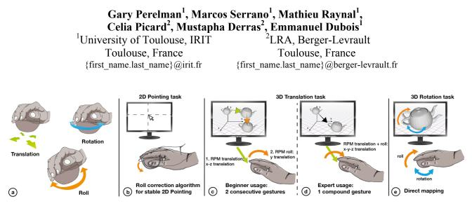
Figure 1.a) The Roly-Poly Mouse (RPM) gestures. RPM can be used for b) 2D pointing; c-d) 3D translation by combining RPM translation and roll; e) and 3D rotation by combining RPM roll and rotation.
