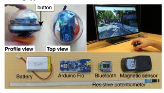
Figure 11. Proof-of-concept wireless prototype with a 'ring' button used in StreetView (top). Components (bottom).
