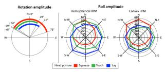
Figure 7. a) Rotation amplitude in degrees for each hand posture; b) rolling amplitude for the Hemispherical version and c) for the Convex version.
