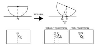
Figure 3. 2D pointing problem with a rolling device.
