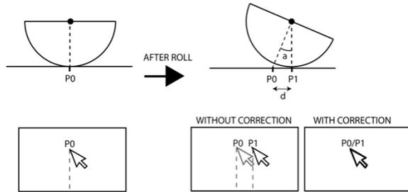
Figure 3. 2D pointing problem with a rolling device.
