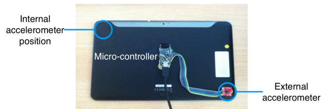
Figure 3. Test prototype with an external accelerometer.
