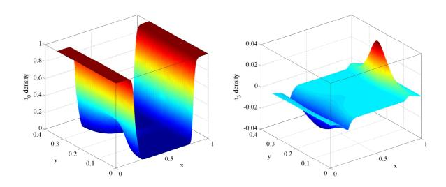
FIGURE 2. Scaled stationary charge density (left) and spin density  $n_3$  (right) in an open-state MESFET with  $V_D = -2$  V and  $V_G = 0$  V.
