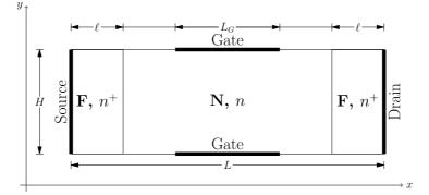
FIGURE 1. Geometry of a MESFET with ferromagnetic (F) source and drain regions and nonmagnetic (N) channel region.
