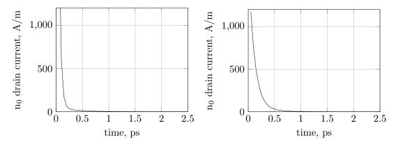
FIGURE 5. Change of the electron drain current in the ferromagnetic (left) and standard (right) MESFET, switching from open to closed state.
