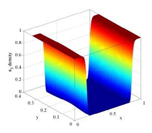
FIGURE 3. Scaled stationary charge density in a closed-state MESFET with  $V_D = -2 \,\mathrm{V}$  and  $V_G = 1.2 \,\mathrm{V}$ .
