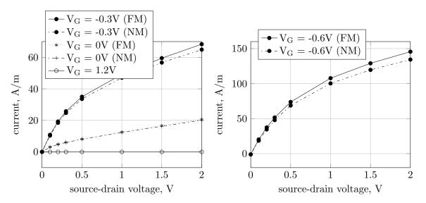
FIGURE 4. Current-voltage characteristics for the ferromagnetic (FM) and standard (NM) MESFET for various gate voltages  $V_G$ . For convenience, the source-drain voltages are given by their absolute values.
