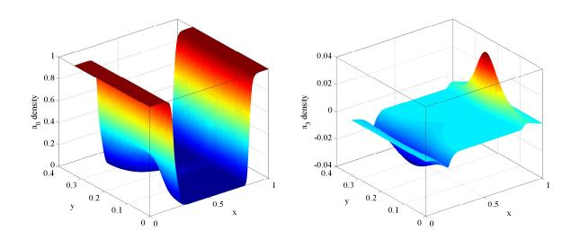
FIGURE 2. Scaled stationary charge density (left) and spin density  $n_3$  (right) in an open-state MESFET with  $V_D = -2 \,\mathrm{V}$  and  $V_G = 0 \,\mathrm{V}$ .
