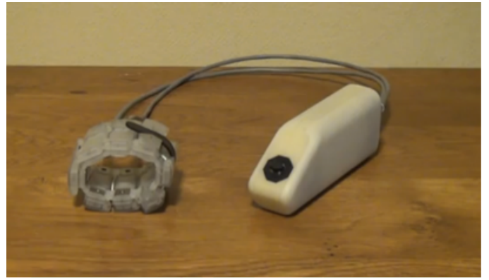
Figure 1. Illustration of the device. Right: Hand-held device ( D_1 ) used to indicate the direction by tilting the small black part. Left: Worn around the wrist ( D_2 ) composed by 8 vibrators.
