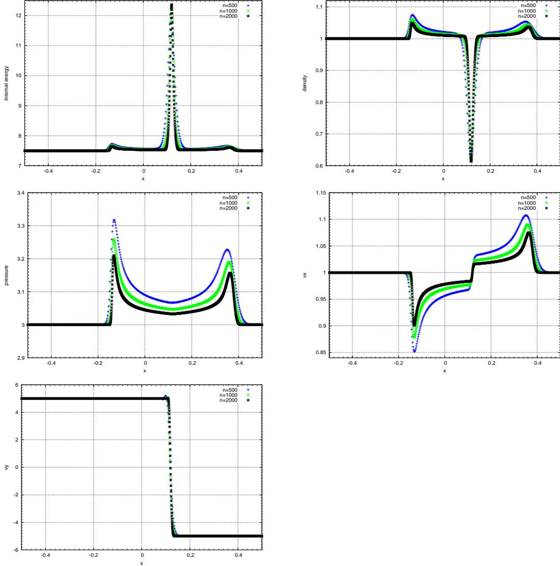
FIG. 17. Slip contact discontinuity – Results for  $h = 1/500$ ,  $h = 1/1000$  and  $h = 1/2000$ , along a line parallel to the x-axis. Internal energy (top-left), density (top-right), pressure (middle-left), x-velocity (middle-right) and y-velocity (bottom).
