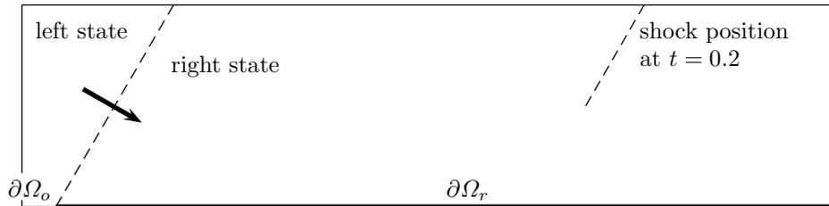
FIG. 9. Double Mach reflection – Geometry and initial conditions.
