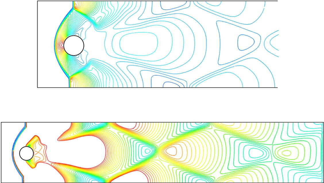
FIG. 15. Mach=10 flow past a cylinder – Top: iso-lines of pressure near the disk ( $p \in (0.0713, 0.957)$ ) at  $t = 5$ ; bottom: still pressure iso-lines but on the whole computational domain, and restricted to the interval  $(0.0713, 0.2)$  (so the areas left in white on the figure correspond to zones where  $p > 0.2$ ).
