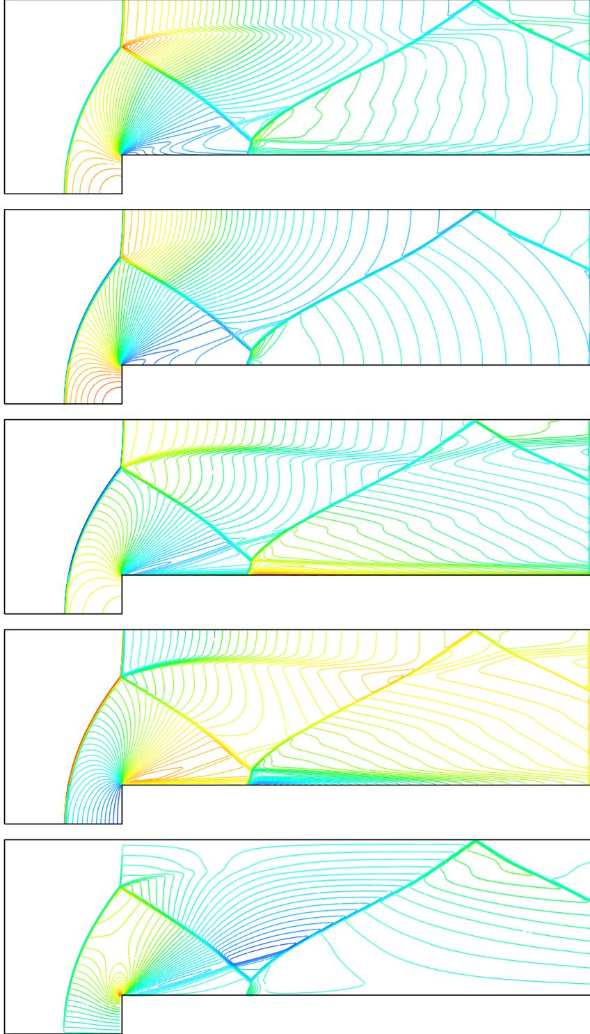
FIG. 8. Mach 3 step – From top to bottom: density, pressure, enthalpy ( $\mathcal{H} = e + p/\rho$ ), first and second component of the velocity at  $t = 4$ , obtained with  $h = 2.5 \times 10^{-3}$ ,  $\delta t = 10^{-3}$  and  $\mu = 10^{-3}$ . The variation intervals of the unknowns are  $\rho \in [0.235, 6.4]$ ,  $p \in [0.216, 12.04]$ ,  $\mathcal{H} \in [2.46, 8.11]$ ,  $u_1 \in [0., 3.046]$ , and  $u_2 \in [-0.92, 1.82]$ .
