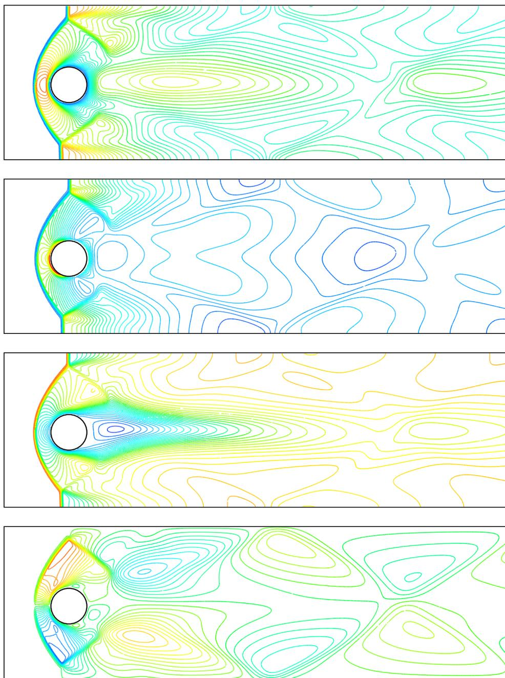
FIG. 16. Mach=10 flow past a cylinder – From top to bottom: internal energy, density,  $x$ -component of velocity,  $y$ -component of velocity at  $t = 5$ . The variation ranges of the unknowns are  $e \in [0.178, 0.536]$ ,  $\rho \in [0.804, 12.23]$ ,  $u_1 \in [-0.11, 1]$ , and the value  $u_1 = 0$  corresponds to the fourth iso-line,  $u_2 \in [-0.326, 0.327]$ .
