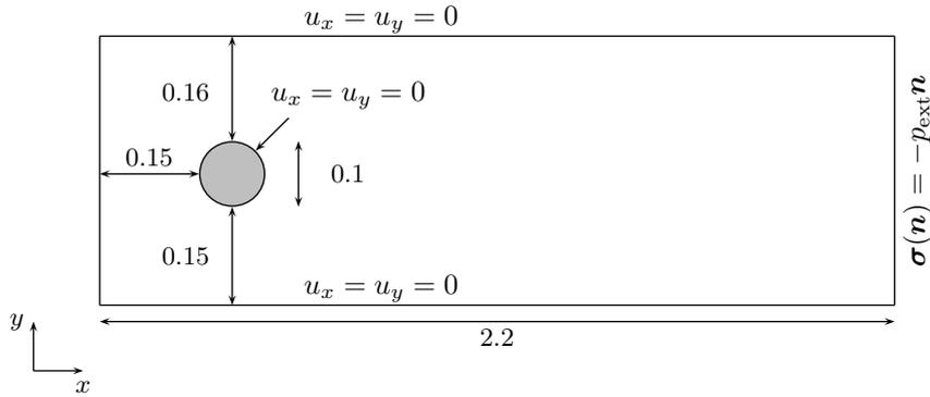
FIG. 13. Low Mach flow past a cylinder – Geometry.
