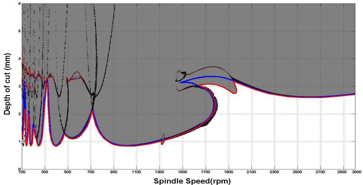
Figure 4. Stability diagram for case 1 comparing ZOA (blue line), combined frequency method (red line) and Multi frequency (shadow zone).
