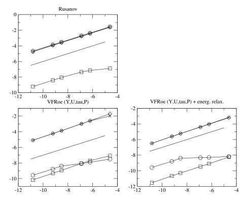
Figure 6: Convergence curves for the test of the section 4.1.2, logarithm of the error (35) versus the logarithm of the mesh size. The meshes contain respectively  $10^2$ ,  $5 \ 10^2$ ,  $10^3$ ,  $5 \ 10^3$ ,  $10^4$  and  $5 \ 10^4$  cells. The circles correspond to the fractions, the square to the density, the diamond to the velocity and the "X" to the pressure. The plain line represents the slope 1/2.
