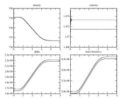
Figure 9: Numerical approximations for the heating pipe test case at time pipe x = 7.316 m versus the time for t = 5 s and for a mesh with  $10^2$  cells. VFRoe-ncv  $(Y, \tau, U, P)$ Plain line: scheme with energy relaxation, dashed line: VFRoe-ncv  $(Y, \tau, U, P)$  scheme
