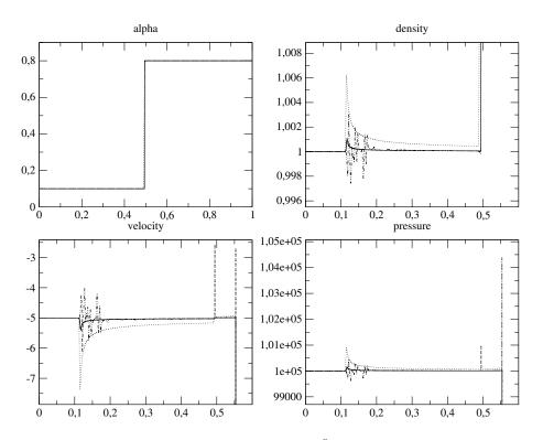
Figure 4: Approximated solutions for  $N=10^5$  obtained with: Rusanov (dot), VFRoe-ncv  $(Y,\tau,U,e)$  (dot-dash), VFRoe-ncv  $(Y,\tau,U,P)$  (dash), and VFRoe-ncv  $(Y,\tau,U,P)$  with energy relaxation (plain line). Zoom on the ghost wave.
