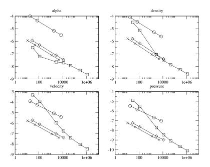
Figure 5: Computational efficiency of the different schemes: error (35) with respect to the CPU time in seconds computed for the meshes  $N = \{5\ 10^3, 10^4, 5\ 10^4, 10^5\}$  and with the additional points  $N = \{2\ 10^5, 5\ 10^5, 10^6\}$  for the VFRoe-ncv  $(Y, \tau, U, e)$  scheme. The circles stand for Rusanov, the squares for VFRoe-ncv  $(Y, \tau, U, e)$ , the diamonds for VFRoe-ncv  $(Y, \tau, U, P)$ , and the crosses for VFRoe-ncv  $(Y, \tau, U, P)$  with energy relaxation.
