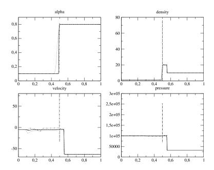
Figure 2: Approximated solutions for  $N=10^3$  obtained with: Rusanov (dot), VFRoe-ncv  $(Y, \tau, U, e)$  (dot-dash), VFRoe-ncv  $(Y, \tau, U, P)$  (dash), and VFRoe-ncv  $(Y, \tau, U, P)$  with energy relaxation (plain line).
