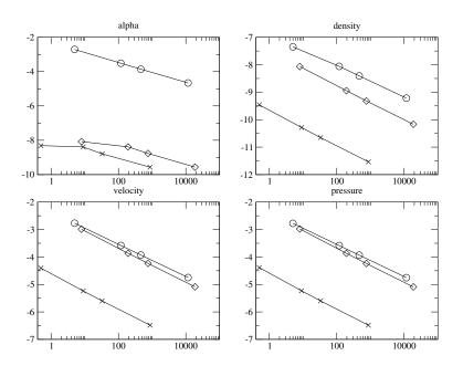
Figure 7: Computational efficiency of the different schemes: error (35) with respect to the CPU time in seconds computed for the meshes  $N = \{10^3, 5 \ 10^3, 10^4, 5 \ 10^4\}$ . The circles stand for Rusanov, the diamonds for VFRoe-ncv  $(Y, \tau, U, P)$ , and the crosses for VFRoe-ncv  $(Y, \tau, U, P)$  with energy relaxation.
