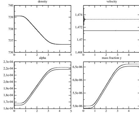
Figure 10: Values at the outlet of the pipe  $x = 7.316$  m versus the time for the heating pipe test case for a mesh with  $10^2$  cells. Plain line: VFRoe-ncv ( $Y, \tau, U, P$ ) scheme with energy relaxation, dashed line: VFRoe-ncv ( $Y, \tau, U, P$ ) scheme
