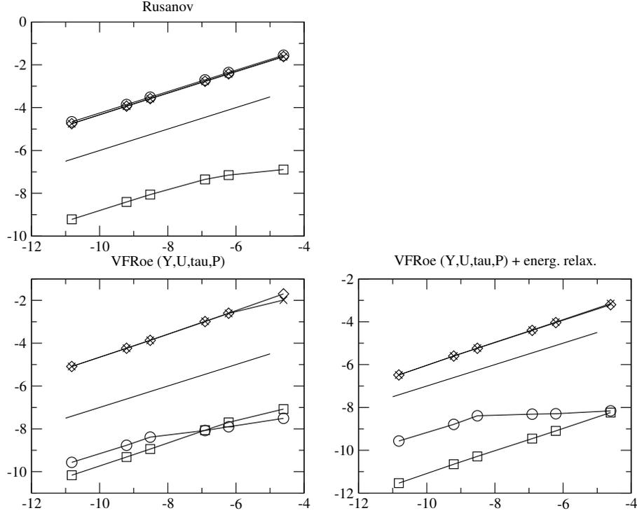
Figure 6: Convergence curves for the test of the section 4.1.2, logarithm of the error (35) versus the logarithm of the mesh size. The meshes contain respectively  $10^2$ ,  $5 \cdot 10^2$ ,  $10^3$ ,  $5 \cdot 10^3$ ,  $10^4$  and  $5 \cdot 10^4$  cells. The circles correspond to the fractions, the square to the density, the diamond to the velocity and the “X” to the pressure. The plain line represents the slope  $1/2$ .
