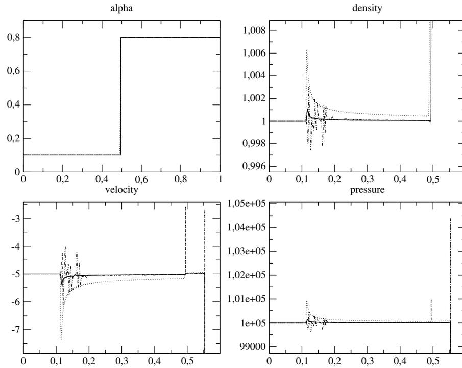
Figure 4: Approximated solutions for  $N = 10^5$  obtained with: Rusanov (dot), VFRoe-ncv ( $Y, \tau, U, e$ ) (dot-dash), VFRoe-ncv ( $Y, \tau, U, P$ ) (dash), and VFRoe-ncv ( $Y, \tau, U, P$ ) with energy relaxation (plain line). Zoom on the ghost wave.
