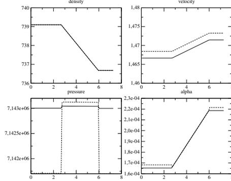
Figure 9: Numerical approximations for the heating pipe test case at time  $t = 5$  s and for a mesh with  $10^2$  cells. Plain line: VFRoe-ncv ( $Y, \tau, U, P$ ) scheme with energy relaxation, dashed line: VFRoe-ncv ( $Y, \tau, U, P$ ) scheme
