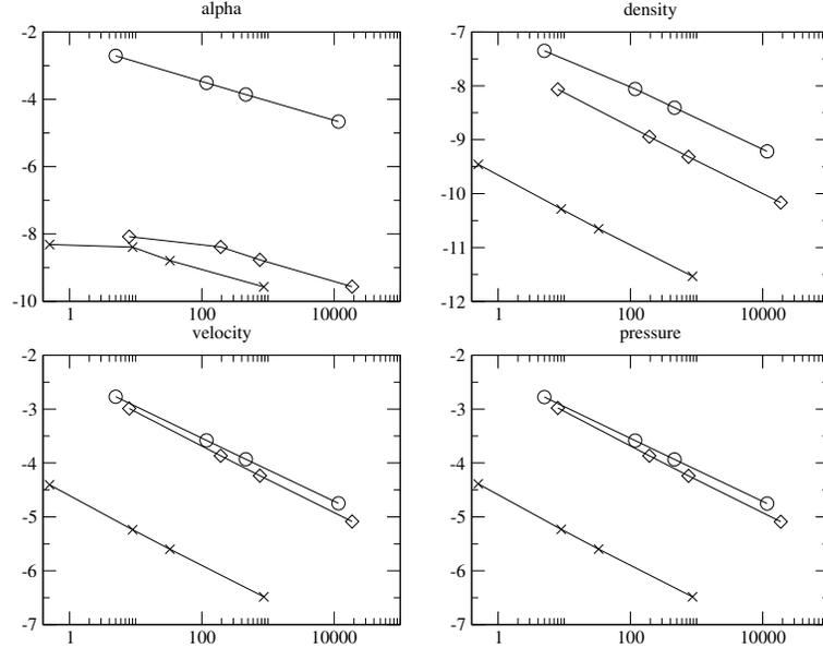
Figure 7: Computational efficiency of the different schemes: error (35) with respect to the CPU time in seconds computed for the meshes  $N = \{10^3, 5 \cdot 10^3, 10^4, 5 \cdot 10^4\}$ . The circles stand for Rusanov, the diamonds for VFRoe-ncv ( $Y, \tau, U, P$ ), and the crosses for VFRoe-ncv ( $Y, \tau, U, P$ ) with energy relaxation.
