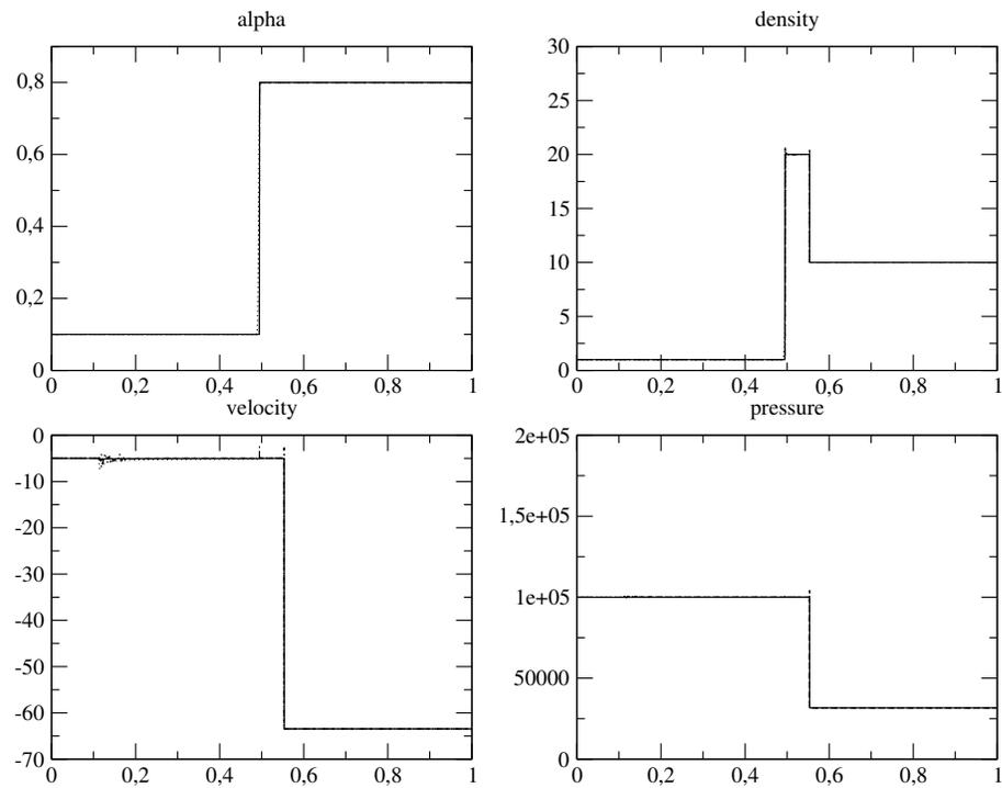
Figure 3: Approximated solutions for  $N = 10^5$  obtained with: Rusanov (dot), VFRoe-ncv ( $Y, \tau, U, e$ ) (dot-dash), VFRoe-ncv ( $Y, \tau, U, P$ ) (dash), and VFRoe-ncv ( $Y, \tau, U, P$ ) with energy relaxation (plain line).
