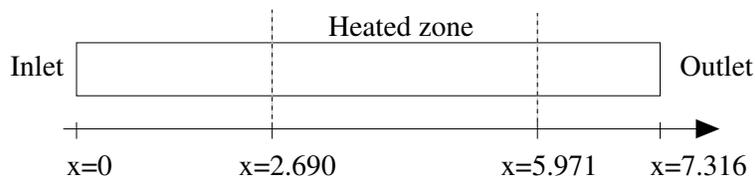
Figure 8: Sketch of the CSNI test case.
