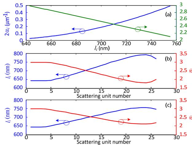
Fig. 2. (a) Calculated required refractive index  $n_i$  of the artificial material of a scattering cell and the corresponding power leakage factor as a function of the cell length  $l_i$ .  $l_i$  and  $n_i$  distributions of the grating couplers designed for coupling to (b) an SSMF and (c) a single core of an MCF.
