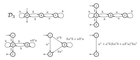
**Figure 3.** The state-elimination method exemplified on the automaton  $\mathcal{D}_3$
