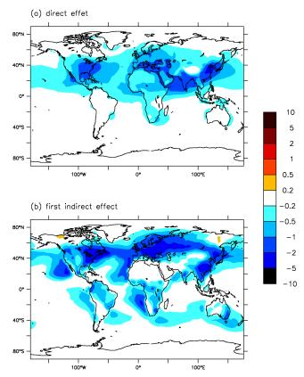
Fig. 4. Radiative forcings (W m<sup>-2</sup>) estimated with the off-line configuration of the model for present-day, sulfate emissions: (a) direct effect (b) 1st indirect effect.
