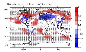
**Fig. 11.** (a) Reference method ( $M_{REF}$ ) radiative forcing of the first indirect effect ( $W\,m^{-2}$ ); (b) difference of radiative forcing between the reference method ( $M_{REF}$ ) and the off-line method ( $CM_{Offline}$ ). The statistical signifiance of the difference was tested at the 95 % confidence level using a bootstrap method. Regions where the difference is statistically significant are indicated with dots.
