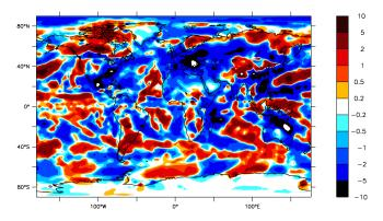
**Fig. 3.** Difference between the short wave top-of-atmosphere net fluxes (in  $W\,m^{-2}$ ) computed with present day and with preindustrial sulfate emissions. The on-line configuration of the model is used.
