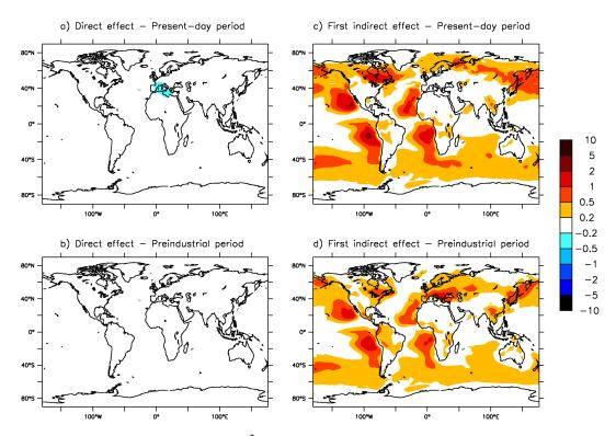
Fig. 6. Difference of the top-of-atmosphere fluxes  $(W m^{-2})$  between the simulation in which the aerosol concentration varies at each time step (VAR experiment) and the simulation in which the concentration remains constant, prescribed to the monthly mean values (MONTH experiment) for present day sulfate emissions (top) and preindustrial sulfate emission (below). Impact of the sulfate first indirect effect (left) and the sulfate direct effect (right) are presented separately.
