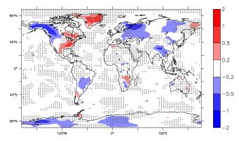
Fig. 12. Impact on surface temperature of coupling chemistry and climate: difference of temperature anomaly ( $\Delta T = T_{\text{PD}} - T_{\text{PI}}$ ) between on-line ( $\Delta T_{\text{V}}$ ) and off-line configuration ( $\Delta T_{\text{M}}$ ). The statistical significance of the difference was tested at the 95 % confidence level using a student test. Regions where the difference is statistically significant are indicated with dots.
