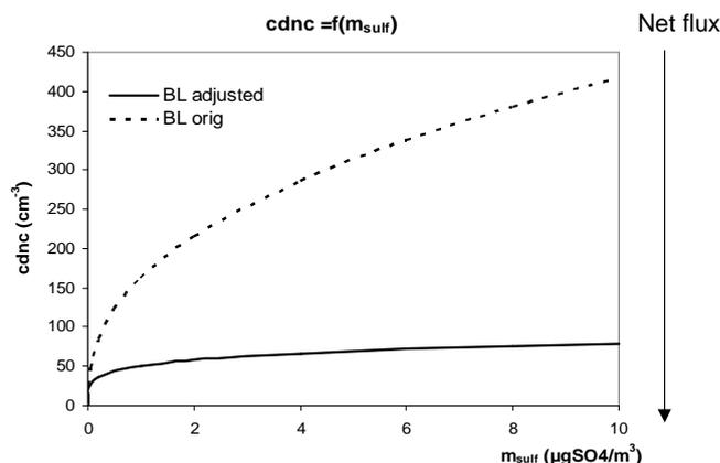
**Fig. 1.** Relationship between clouds droplet number ( $\text{cm}^{-3}$ ) and the sulfate concentrations ( $\mu\text{gSO}_4 \text{m}^{-3}$ ) from the Boucher and Lohmann (1995) D formula, with the original empirical constant (dashed) and with the adjusted empirical constant of Quaas and Boucher (2005) (solid line).
