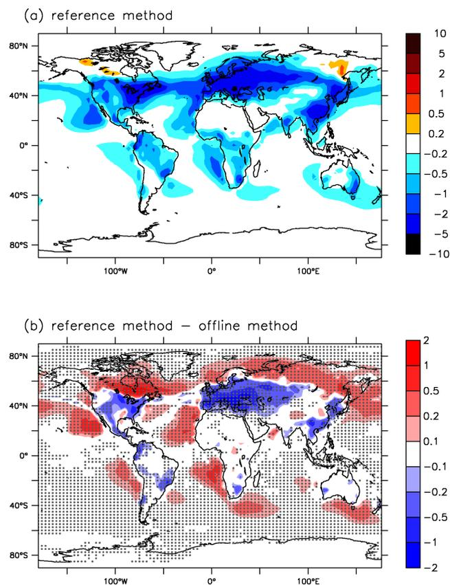
**Fig. 11.** (a) Reference method ( $M_{\text{REF}}$ ) radiative forcing of the first indirect effect ( $\text{W m}^{-2}$ ); (b) difference of radiative forcing between the reference method ( $M_{\text{REF}}$ ) and the off-line method ( $CM_{\text{Offline}}$ ). The statistical significance of the difference was tested at the 95 % confidence level using a bootstrap method. Regions where the difference is statistically significant are indicated with dots.
