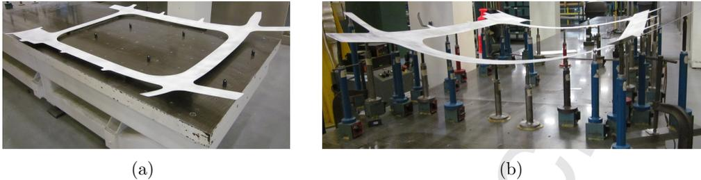
Figure 2: Example of an aerospace panel: (a) in a free-state, (b) mounted on its inspection fixture before the measurement process. (source: Bombardier Aerospace)
