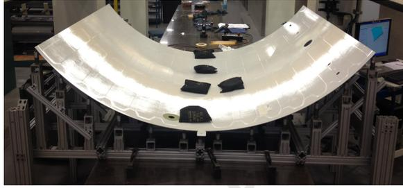
Figure 1: Example of an aerospace panel restrained by known forces (i.e., using weights) on its inspection fixture. (source: Bombardier Aerospace)
