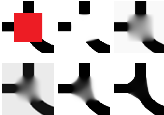
FIGURE 8. Top row: Damaged image and restored ones using total variation and harmonic models, respectively. Bottom row: Restored images using biharmonic model and our approach at iterations 5 and 20, respectively.
