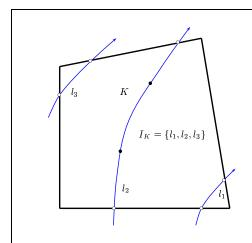
Fig 1. Streamline path throught grid cell K
