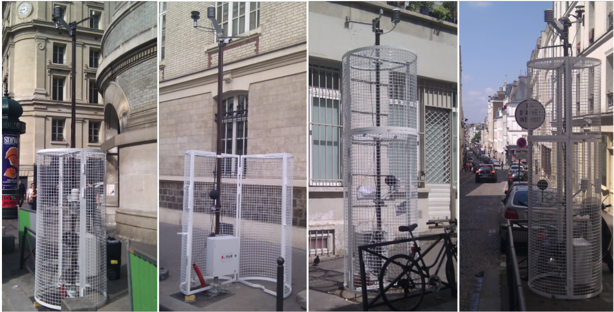
Figure 4: Photographs of weathered and control weather stations in situ, from left to right : weathered and control Louvre stations, weathered and control Belleville stations.
