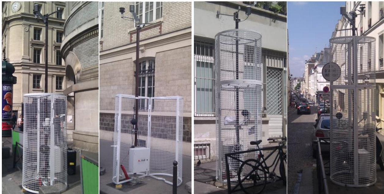
Figure 4: Photographs of watered and control weather stations in situ, from left to right : watered and control Louvre stations, watered and control Belleville stations.
