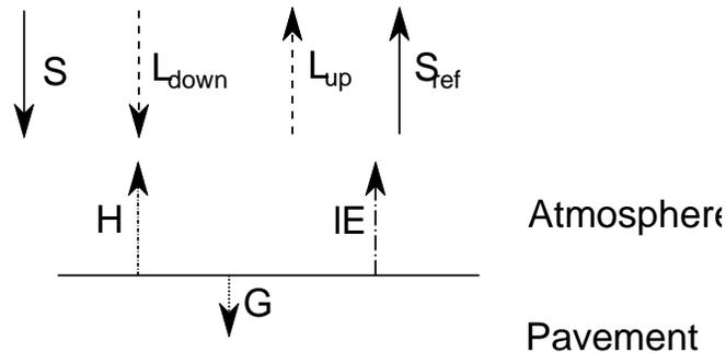
Figure 6: Diagram of pavement heat budget at surface
