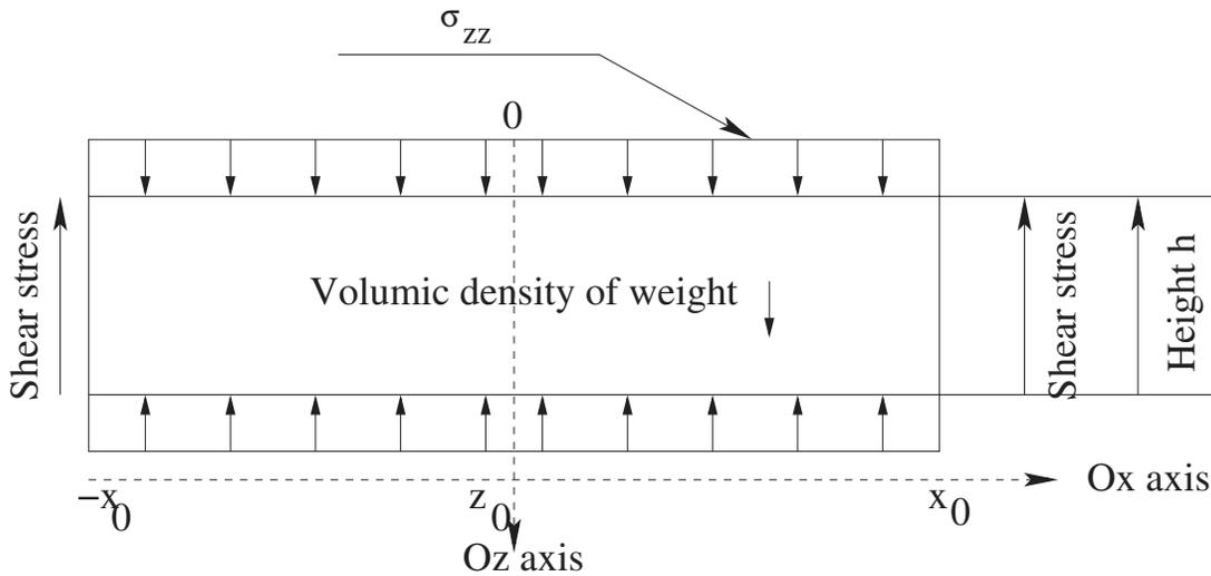
**Figure 2.** Representation of a slice of ensiled matter
