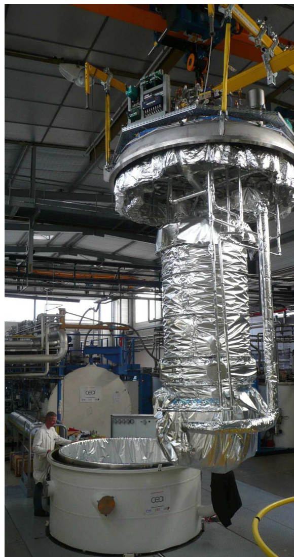
FIG. 8. Insertion of the saturated bath (covered with MLI) into the Multipurpose cryostat.
