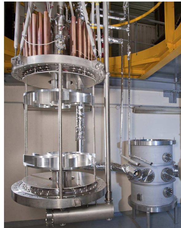
FIG. 3. The von Kármán experiment with top and bottom flanges, upper and lower propellers (left) and its outer chamber with ports (right). Copper heat exchangers can be seen (upper left).
