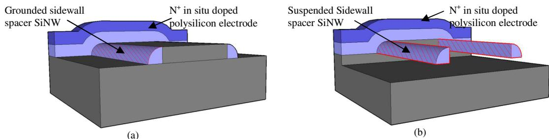
Fig. 2: Schematic view of grounded (a) and suspended (b) sidewall spacer polycrystalline SiNWs based resistors
