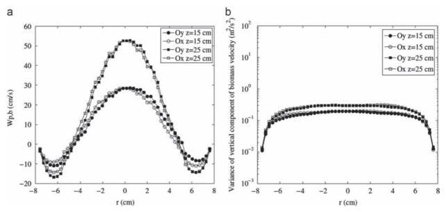
**Fig. 16.** (a)Time-averaged and (b) variance of the vertical component of biomass velocity in two perpendicular directions as obtained from the 3-D numerical simulation (biomass fraction: 8 wt%,  $U/U_{mfs}$ =4).
