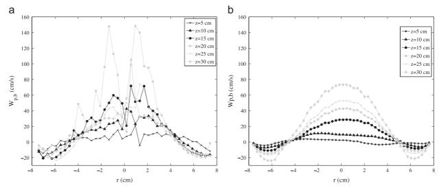
**Fig. 13.** Comparison between (a) the RPT experimental measurements and (b) the 3-D numerical simulation results for the time-average vertical component of biomass velocity. (biomass fraction: 8 wt%,  $U/U_{mf,s}$ =4).
