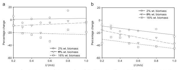
**Fig. 3.** Percentage change of mean bubble size vs. superficial gas velocity for sand fluidized beds involving different loads of (a) spherical and (b) cylindrical biomass particles with reference to a bed of pure sand (h=175 mm, r/R=0).
