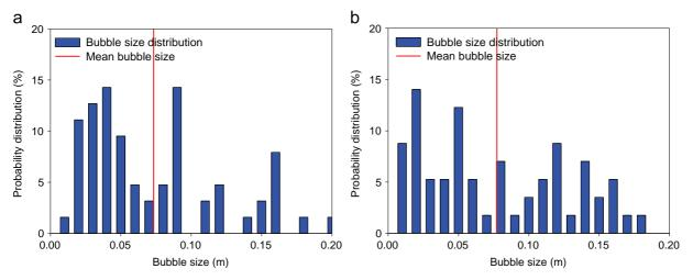
**Fig. 7.** Comparison of (a) experimentally measured and (b) numerically calculated bubble size distribution for the mixture composed of 8 wt%. spherical biomass particles  $(U/U_{mf,s}=4, r/R=0, h=175 \text{ mm})$ . Red lines indicate the mean value of the bubble size (For interpretation of the references to color in this figure legend, the reader is referred to the web version of this article.)
