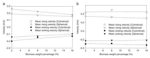
**Fig. 4.** Mean rising and sinking velocities of the biomass particle involved in gross circulation for systems fluidized at (a)  $U/U_{mfs}$ =2 and (b)  $U/U_{mfs}$ =3.6 for cylindrical and  $U/U_{mfs}$ =4 for spherical biomass particles.
