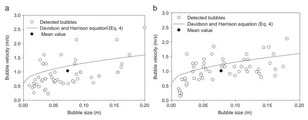
**Fig. 9.** The rise velocity of all detected bubbles vs. the respective sizes for the mixture composed of 8 wt% spherical biomass particles as obtained from (a) experiments and (b) simulation  $(U/U_{mf,s}=4, r/R=0, h=175 \text{ mm})$ . Full black dots denote the mean bubble rise velocity vs. the mean bubble size. The solid curve represents the Davidson and Harrison equation (Eq. (4)).
