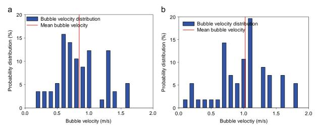
**Fig. 8.** Comparison of (a) experimentally measured and (b) numerically calculated bubble velocity distribution for the mixture composed of 8 wt% spherical biomass particles ( $U/U_{mf,s}$ =4, r/R=0, h=175 mm). Red lines indicate the mean value of the bubble velocity (For interpretation of the references to color in this figure legend, the reader is referred to the web version of this article.)
