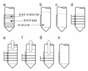
Fig. 1. Schematic presentation of the "frozen bed" technique.
