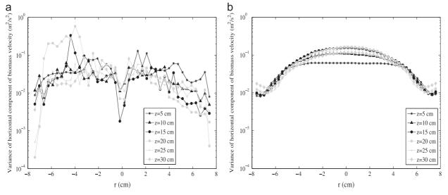
**Fig. 15.** Comparison between (a) the RPT experimental measurements and (b) the 3-D numerical simulation of the variance of the horizontal component of biomass velocity. (biomass fraction: 8 wt%,  $U/U_{mf,s}$ =4).
