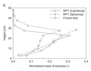
**Fig. 5.** Axial profile of the normalized mass of biomass as obtained by the RPT and frozen bed techniques for mixtures fluidized at  $U/U_{mf,s}$ = 3.6 for cylindrical and  $U/U_{mf,s}$ = 4 for spherical biomass particles, which are composed of (a) 2 wt% (b) 8 wt % and (c) 16 wt%.
