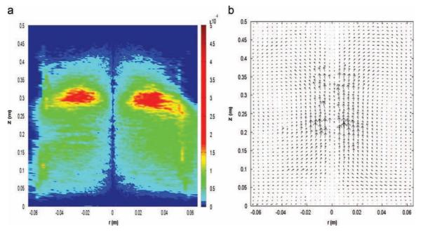
**Fig. 12.** (a) Time-average concentration (occupancy) and (b) velocity profile of the biomass particles in the entire bed as obtained from the RPT experiments. (biomass fraction: 8 wt%,  $U/U_{mf,s}$ =4).
