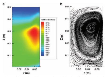
Fig. 11. (a) Time-average volume fraction and (b) streamline of the biomass particles in the bed as obtained from the numerical simulation. (biomass fraction: 8 wt%,  $U/U_{mf,s}$ =4).
