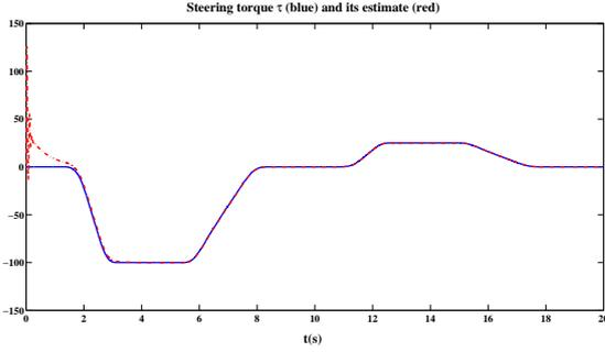
Fig. 2. Rider's torque (blue) and estimated torque (red)
