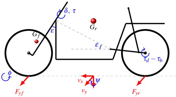
Fig. 1. Geometrical representation of the Sharp's motorcycle model
