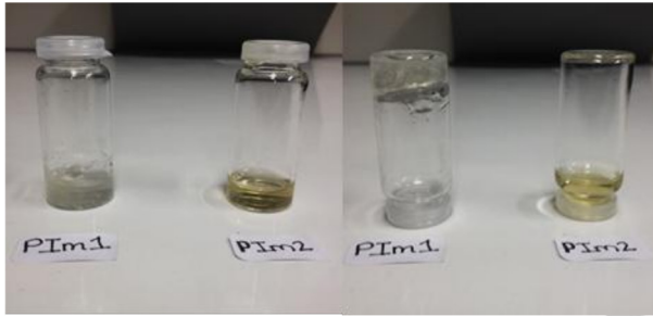
Figure 2: Pictures of 10% weight solutions of PIm1 and PIm2 in water before (left) and after (right) flipping of the vial.
