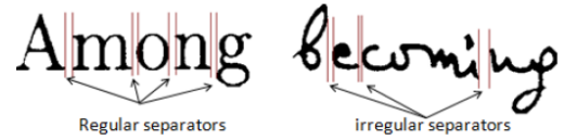
Fig. 2. Separator length between two successive connected components.
