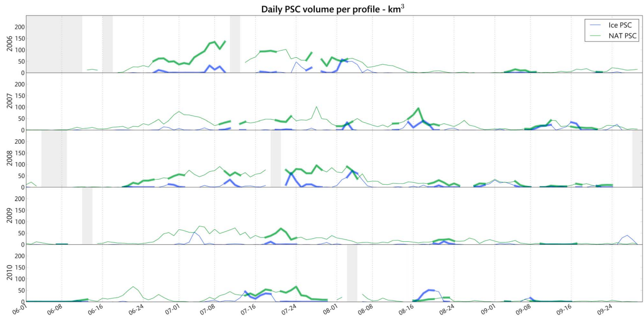
Figure 8. Evolution of PSC volume per profile along each Antarctic winter between 2006 and 2010, for ice (blue) and NAT (green) PSC. Thick lines indicate periods identified as GW events following Table 1. Shaded regions indicate undersampled periods (e.g., missing CALIOP observations).
