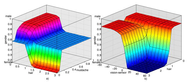
Figure 14: Surface view of input and output variables. a) Relation of the hair, mustache and gender. b) Relation of the vision-sensor, hair and gender.
