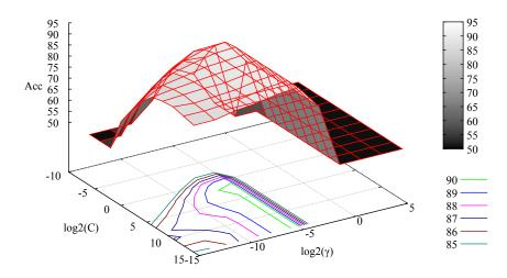
Figure 9: SVM+RBF parameter space and corresponding five-fold cross-validation accuracy for GENKI-4K. Selected parameters C = 4 (log<sub>2</sub>(C) = 2) and  $\gamma = 0.03125$  (log<sub>2</sub>( $\gamma$ ) = -5).
