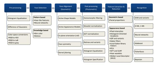
Figure 1: General processing chain for 2D-FGR methods.
