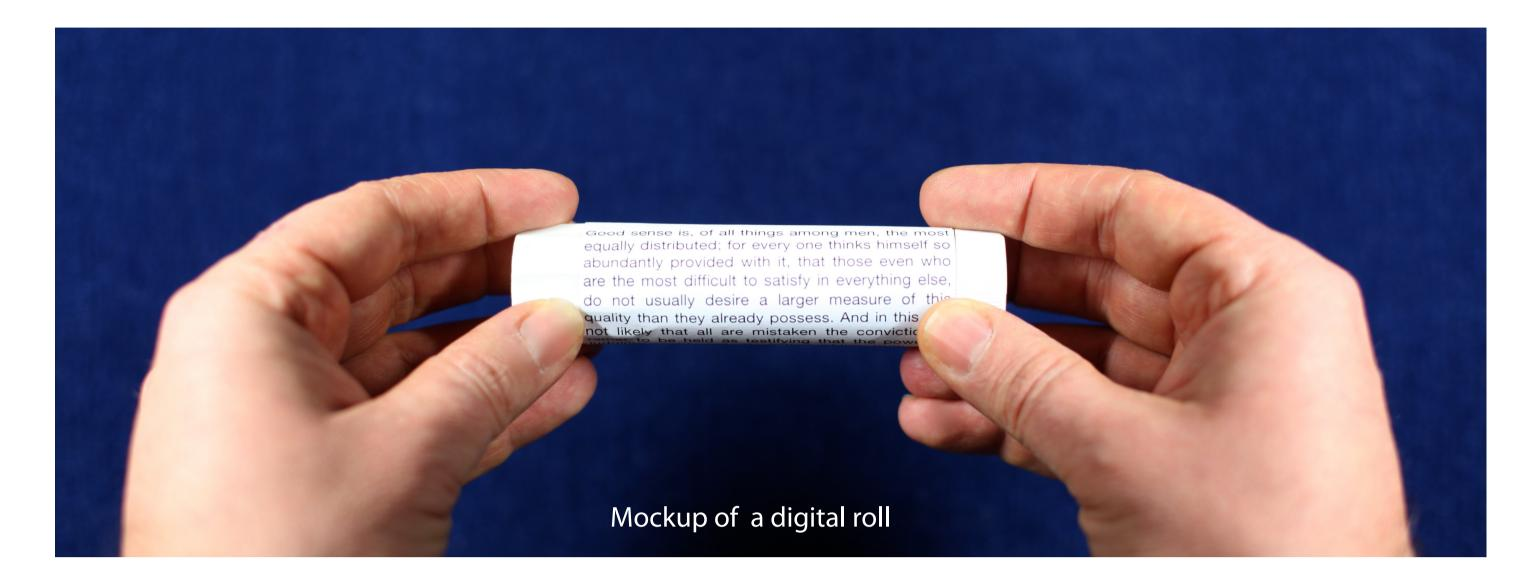
We introduce the Digital Roll, a cylindrical e-reader with a curved display wrapped around it. The device is designed for recreational reading on the go. We investigate a display metaphor illustrated by the mock-up above, where text is glued on the tube and scrolling is performed by manual rotation of the whole device.
