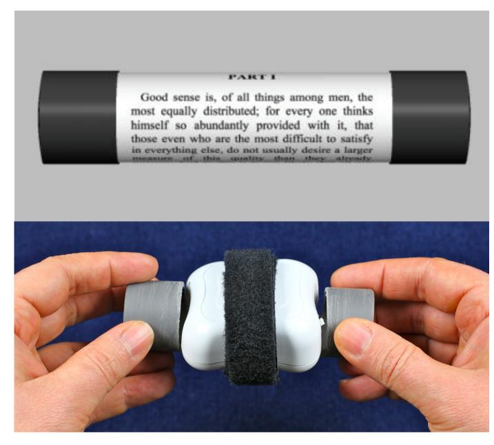
Top: 3D rendering of the roll Bottom: Intersense IMU encased in PVC tube
