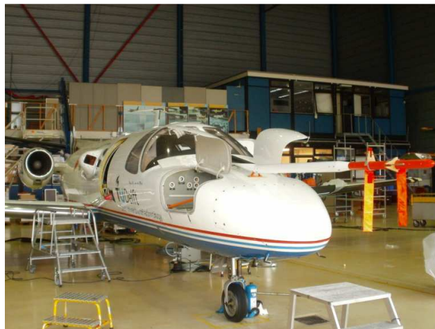
Figure 12: Modified Citation including nose boom and fairing
