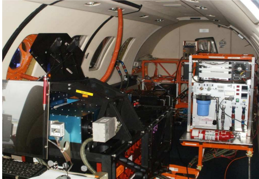
Figure 9: DELICAT equipment installed inside cabin of Cessna Citation II
