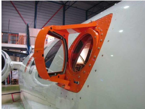
Figure 11: UV optical window with mounted forward reflecting mirror
